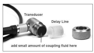
The transducer must be used correctly in order for the TI-007 to produce accurate, reliable measurements. Below is a short description of the transducer, followed by instructions for its use.
